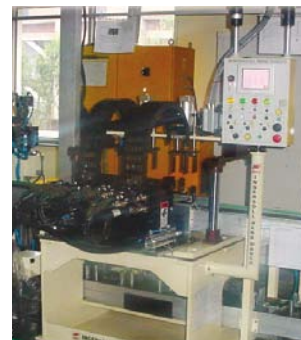
8 Spindle Machine Mounted DC Nutrunner for Fully Automated Operation (tact time = 6 sec.) for Compressor Head Tightening
