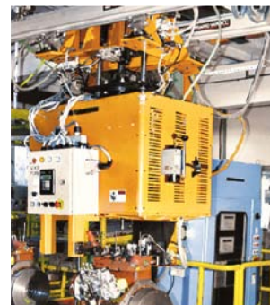
Single Spindle with Servo Controlled X-Y Axis Movement for Auto Sequenced Tightening of Cylinder Head
