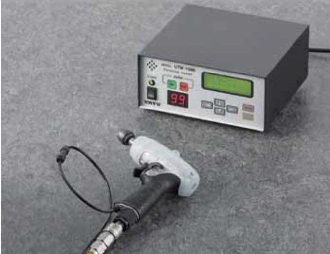
UTM-1500(PS): Pressure Sensor Incorporated type By connecting the TM signal hose from a tool to the coupler at the back of the controller, the pressure sensor incorporated in the controller converts the air pressure signal into the electric signal.
