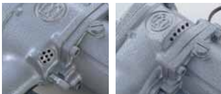
Front exhaust type (model which does not have "R" in model name.)
