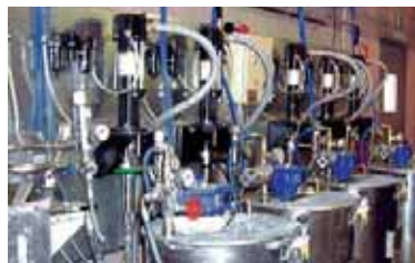
2-ball piston pumps 11:1 ratio, used in a painting circulating system
