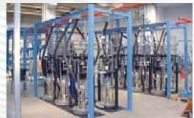
Large extrusion piston pumps, 13:1 ratio, installed on an offset ink formulation system process
