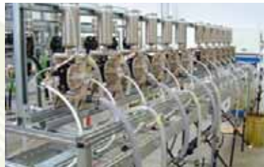
1/2" diaphragm pumps assembled in an ink formulation system
