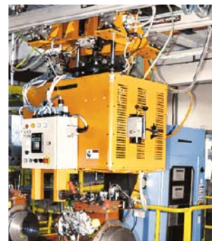
Single Spindle with Servo Controlled X-Y Axis Movement for Auto Sequenced Tightening of Cylinder Head
