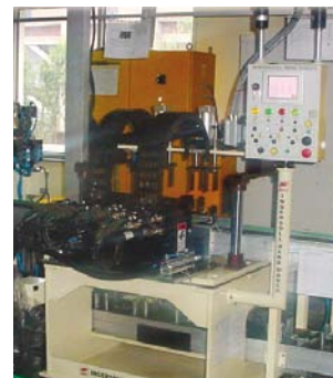
8 Spindle Machine Mounted DC Nutrunner for Fully Automated Operation (tact time = 6 sec.) for Compressor Head Tightening
